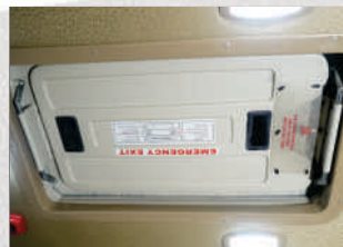
Two Emergency Exit Roof Hatches
